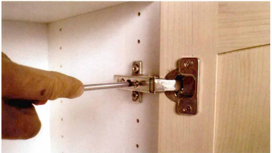
Hinges are adjustable. Slots in the hinge-mounting plates allow the hinge to be moved in and out, and up and down, which makes it easy to get the door to lay flat, square and centered on the cabinet.
